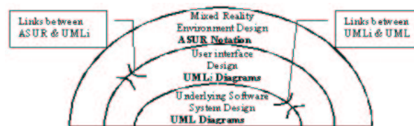
Fig. 4. Layers playing a role in AR systems design and candidate-tools to support these layers.
